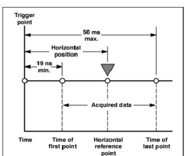
Refer to the illustration below for a diagram of the relationships of time of last point, time of first point, horizontal position, and horizontal reference point.
